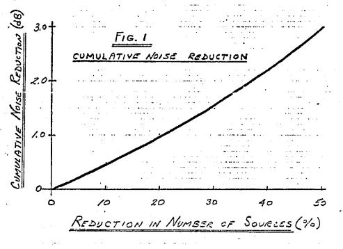
Figure 1 indicates that if 8 aircraft, each generating the same level of noise, produced a cumulative noise level of 110 EPNdB, 4 of these aircraft would then produce a cumulative noise level of approximately 107 EPNdB.
